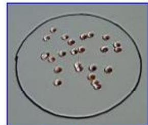
Sample1 Post Test Impact Side Closeup
